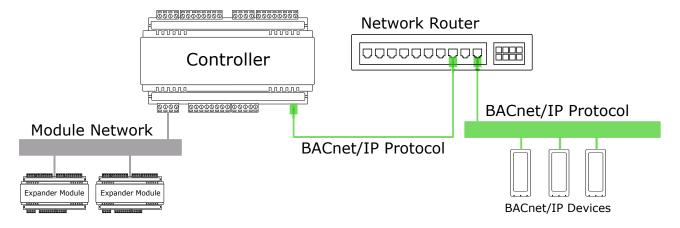
Protege GX modules communicate with the controller on the Protege GX module network as normal, independently of the BACnet network.
