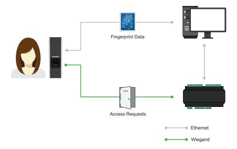
Biometric devices can be used on their own for door and area access, which is convenient for end users as they always have their credentials on hand. For added security, combine biometric devices with ICT card readers to provide dual factor authentication alongside a card or PIN code.
