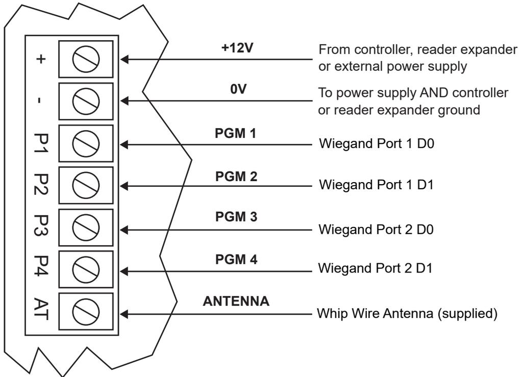
When the receiver is integrated with an access control system, the 0V terminal must be connected to the ground of the controller or reader expander to provide a reference for the Wiegand signals. If the receiver is powered by an external power supply, it must be connected to the controller/expander ground as well.
